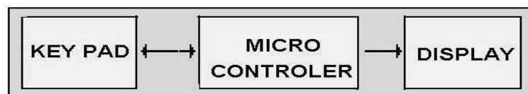
Fig: Interfacing Key Board to 8051.
